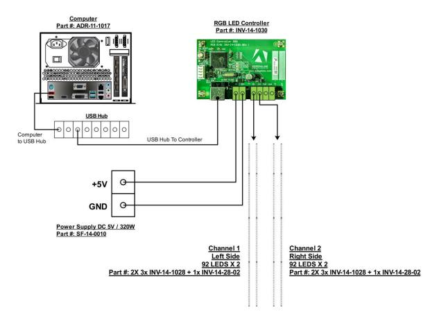
Each side has 2 strips of RGB PCB LED assembly. (Ref p.26) Each strips has 3x 25LEDs PCB (INV-14-1028) and 1x 17LEDs PCB (INV-14-1028-02)
